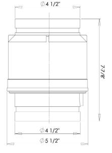
6510210BR: 4" groove x groove spring loaded check valve
