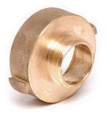
Forged brass reducing adapter that changes the size and/or thread configuration. The female thread is larger than the male thread and will come with either pin lug or rocker lug.
