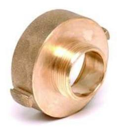
Used to reduce fire hose threads. Female thread is larger than male thread. Also used to change fire hose threads. Specify regional hose threads at time of order. Comes in both Pin Lug and Rocker Lug.
