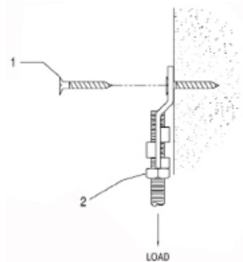
1. Screw hanger directly into structure.
