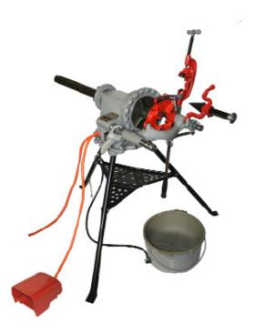
PT<sup>®</sup> Reversible 1/2 HP universal motor. Capacity: 1/8"-2" (3mm-50mm) pipe On/Off/Reverse switch.
