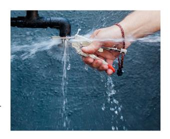
The Quickstop Commercial Tool is the ONLY sprinkler tool on the market that stops ½" and ¾" heads whether they are intact, damaged or completely sheared off.
